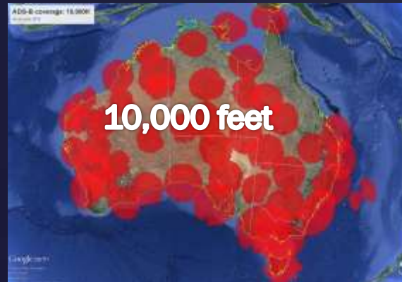
ADS-B Coverage in Australia at Altitudes Used by GA (source: Airservices Australia)
