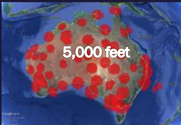
ADS-B Coverage in Australia at Altitudes Used by GA (source: Airservices Australia)
