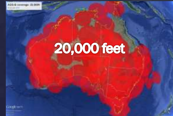
ADS-B Coverage in Australia at Altitudes Used by GA (source: Airservices Australia)
