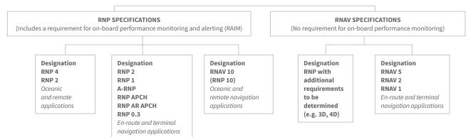
The numerical designators define the level of accuracy required of the navigation system, for example RNP 2 should accurately pinpoint the aircraft to within two nautical miles, 95 percent of the time.
